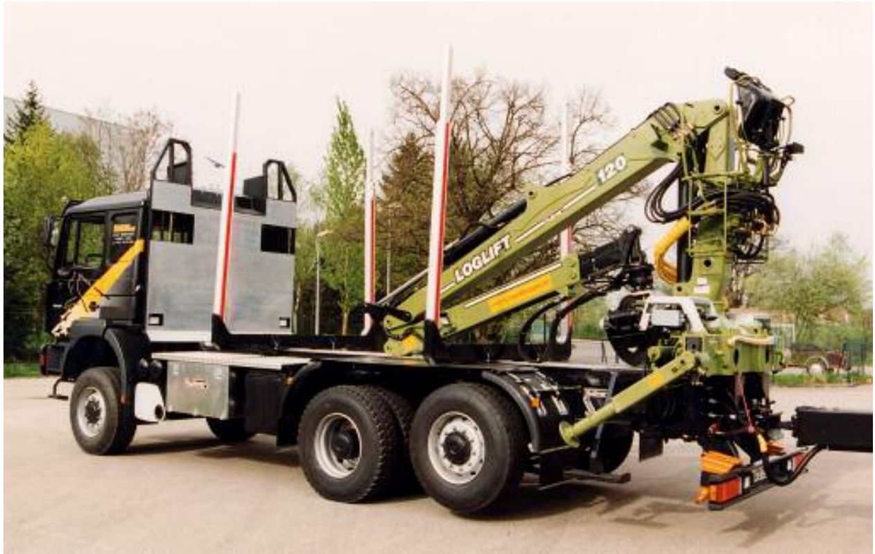
MAN 28.464 (6x4) + NL+ Liftachse + Loglift F 120S
